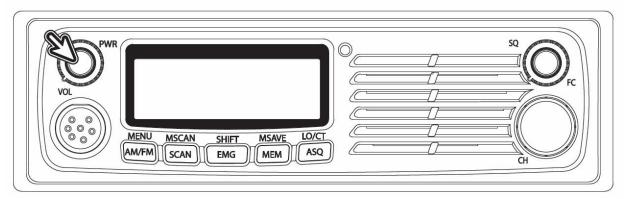
Turn the rotary volume switch clockwise to power on and adjust the sound level for comfortable reception.
