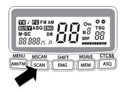
Now the radio scans automatically only the memorized channels and stops where radio traffic is detected.
